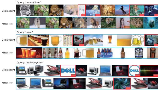
Fig. 4. Ranking comparison on the training data. For each query, top 10 images are returned. The upper ranking list is simply sorted by the click count of the query-image pairs (which may be noisy) and the lower list is sorted by the cosine similarity of the learned representation between the query and the images. The images in red indicate that the images may be irrelevant to the corresponding query.
